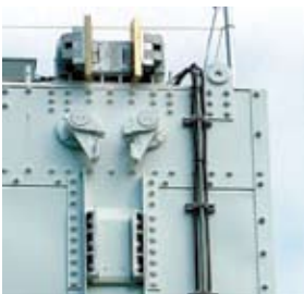
Top: 128 Man Double Deck Aluminum / Steel cage with re-moveable intermediate floor, Aluminum Inspection Hood, Hydraulic Chairing Device, Safety Dogs and Guide Rollers
