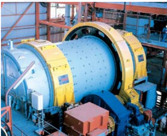
Shell Supported SAG Mill Kopanang Gold Plant, South Africa (4,9 m 9,15 m dia.)
