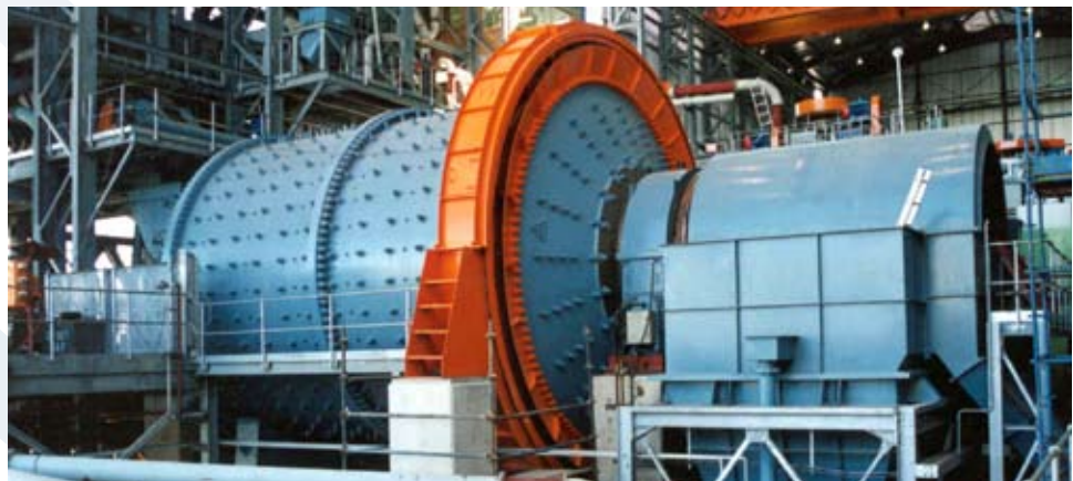
SAG Mill at Amandelbult Platinum Mine, South Africa (6,1m x 8,2m dia)
