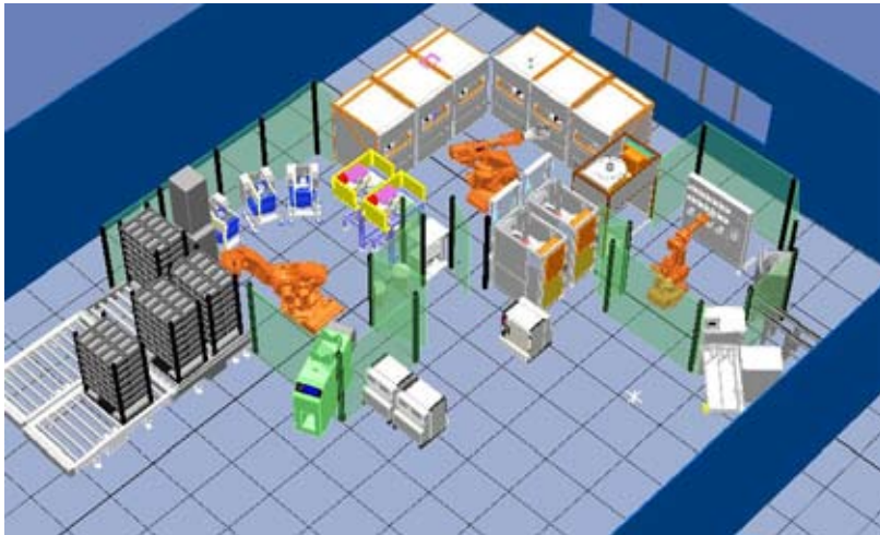
QCX software controls this automated laboratory with its sample infeed, coarse sample preparation, milling and splitting and fire assay dosing cells
